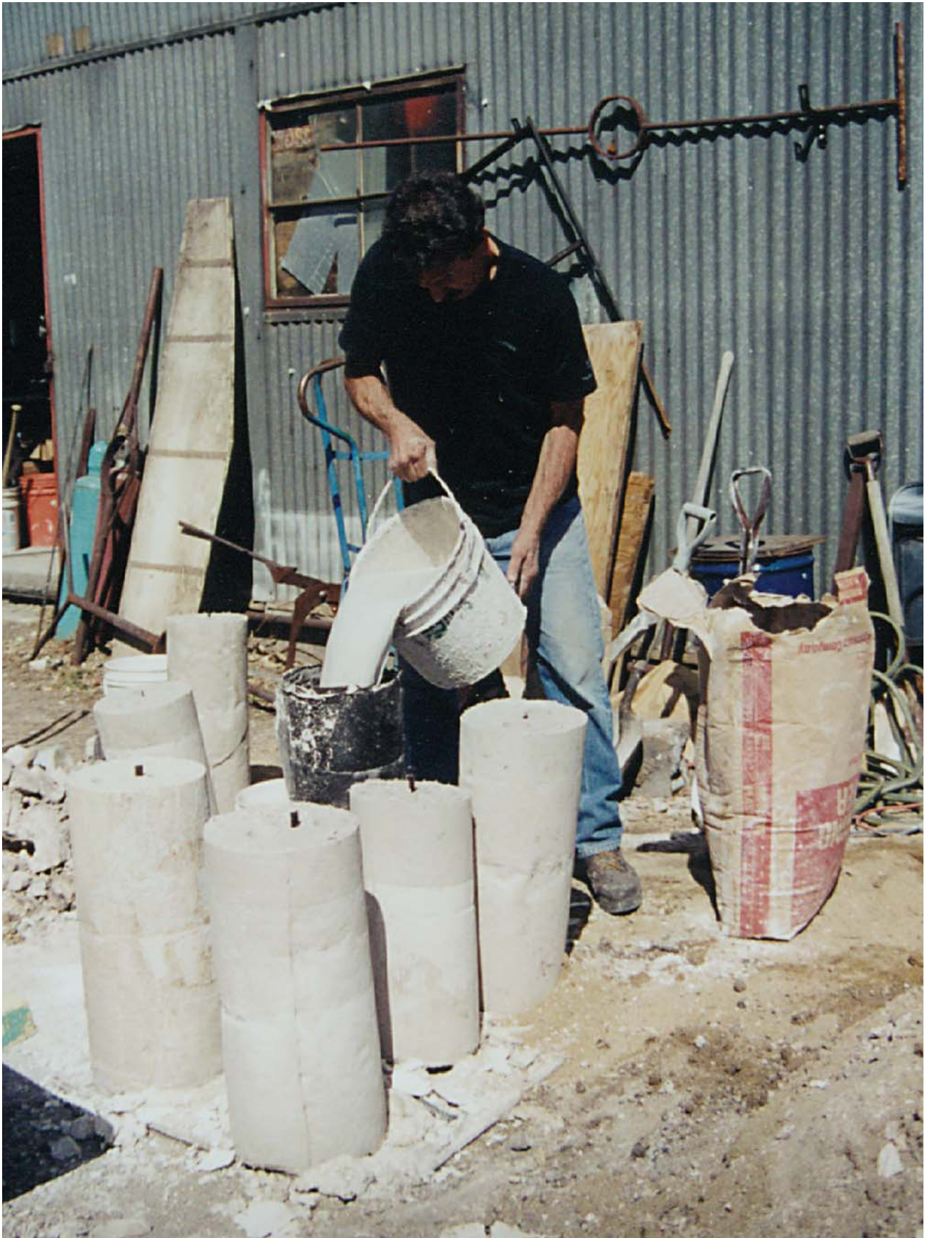
Making investment molds; each contains wax sculptural sections.
