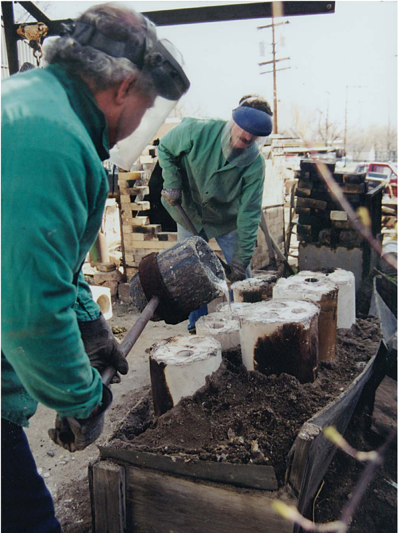
Pouring molten metal into burned-out molds.
