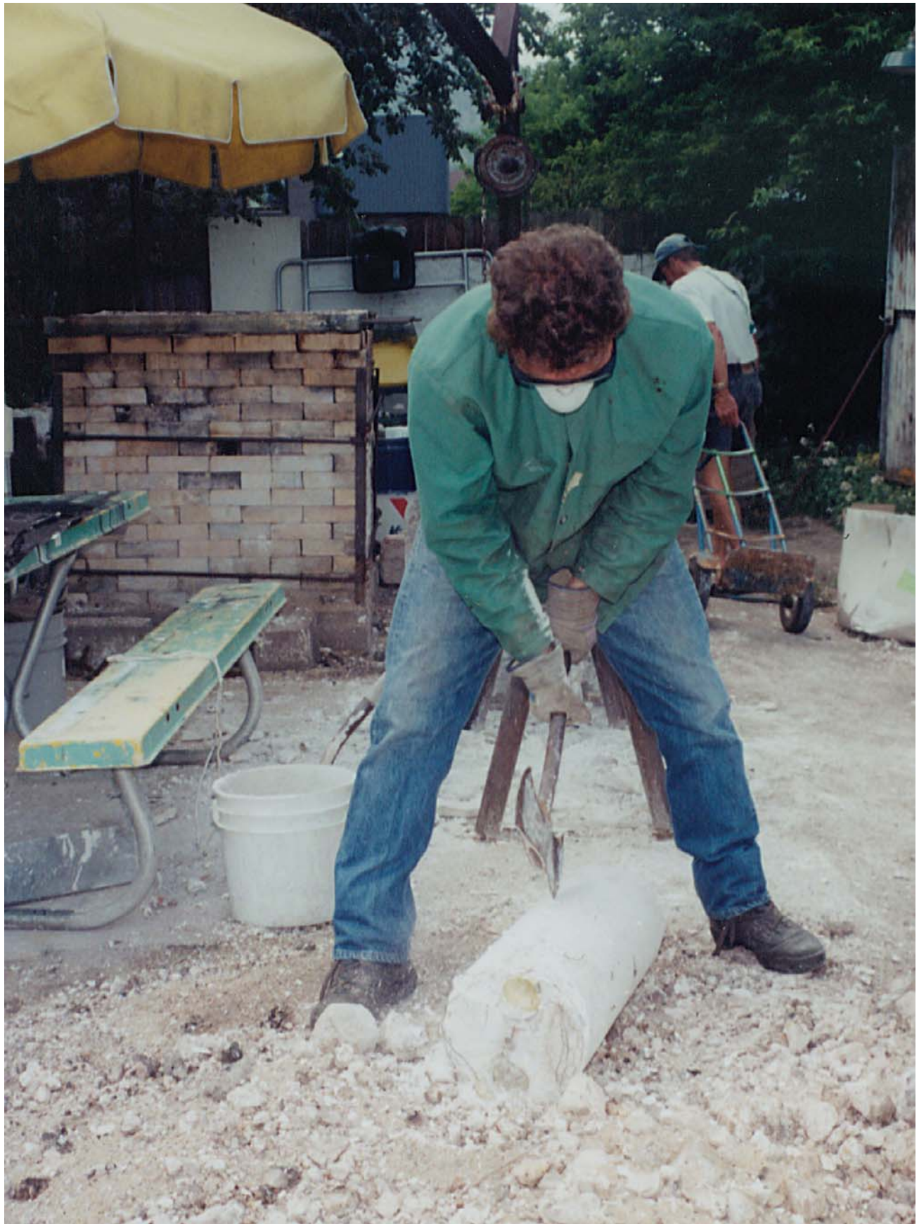
Breaking open molds that contain metal sculptural sections.
