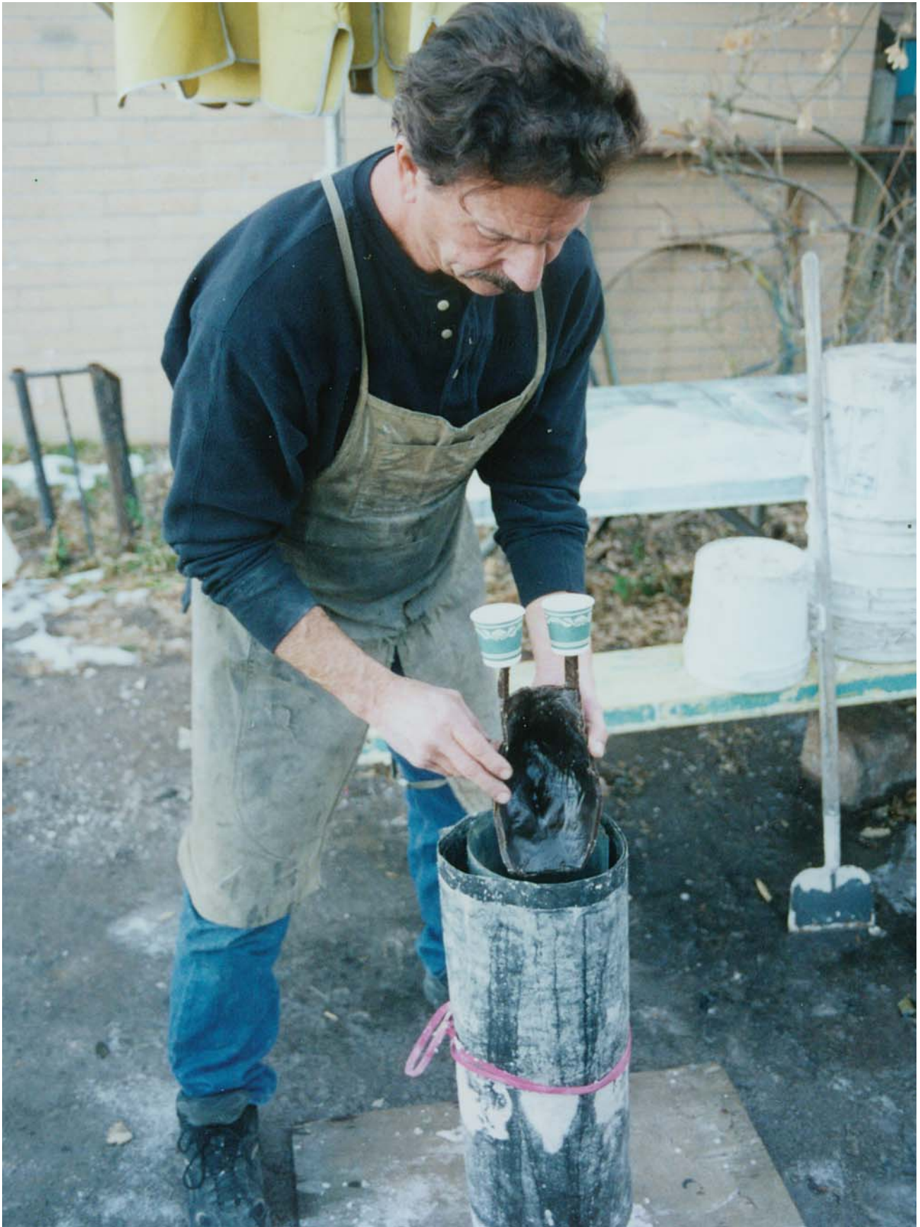
Placing wax sculptures into mold cylinders
