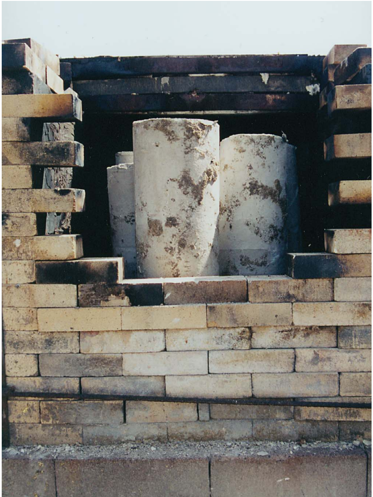
Molds in kiln to be burned out.
